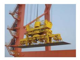
Prior to every lift, the SGM patented Flux Measuring Device FMD checks the lifting safety conditions under which the electro-permanent magnet is working (contact conditions between surface of the load and magnet polarities).
