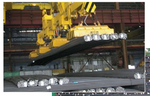
The use of magnets allows for the easy storage of bundles in tidy stacks with no limit in man height or truck height and no need for walkways between stacks. The result is better use of customer's storage volume.
