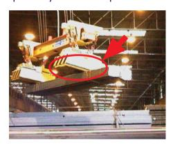
At AFV Beltrame a short beam with no. 2 electromagnets is used for handling bundles up to 6 metres in length whereas a long beam with no. 4 electro-magnets is used for handling bundles up to 14 metres in length.
